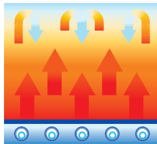
... surface regulation systems provide even heat / chill output which prevents dust turbulence from the offset.
