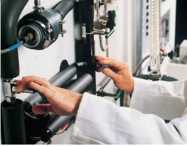
Continuous measurements on the oxygen impermeability of Hewing PE-Xc pipes for heating applications show they are well within limit values specified in DIN.
